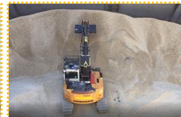
Remote Control Loading
