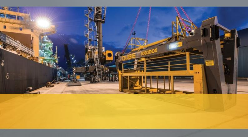
Qube pioneered the design and development of rotating container tippers with integrated lid lifters, revolutionising the way bulk ores and concentrates are transported and loaded.
